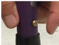
**Moving wheel lock from right side (default) to left:** The wheel lock is useful when getting into or out of the LifeGlider, to prevent it from rolling. If you wish to move the wheel lock handle from the right side to the left, unscrew the bolt holding it in place, move to the left handle, and re-tighten the bolt.
