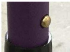
To adjust the device height, identify the adjustment button on the legs. Adjust one leg at a time by pressing in firmly on the adjustment button to release. Then slide the leg to the desired height, and ensure the button fully protrudes from hole corresponding to new height setting. Make sure all legs are set to the same height.
